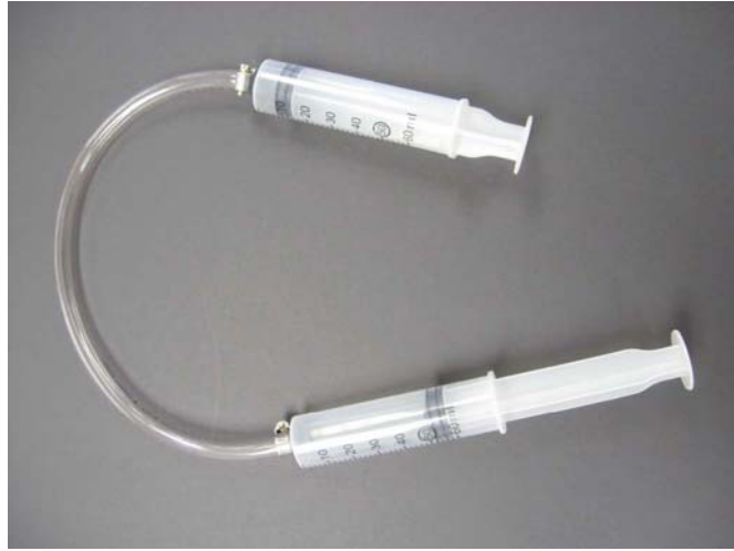
Figure 1. The "Sealed-Syringe" demonstration device. A fixed amount of air is enclosed in the system such that depressing one plunger results in opposite plunger extending. Students will also be asked to press both plungers down simultaneously, compressing the air inside the system which is another conceptual aspect of the interviews.
